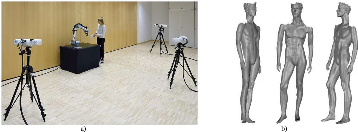
Figure 4: a) Human-machine interface (HMI) usage scenario: A technician presents a part to a robot-based scanning station. b) Three views of a 3D model, simultaneously acquired by three full-resolution 10 Hz 3D sensors (1.0 m x 2.0 m x 0.5 m).
