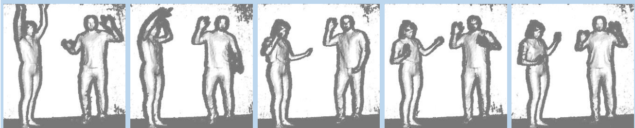
Figure 5: Measurement results from a \geq 10 seconds dynamic performance scene: Two actors play simultaneously on virtual music instruments. The 3D data was recorded with the frontal scanner at 100 fps 2D (20 fps 3D) rate using 2x2 binning.
