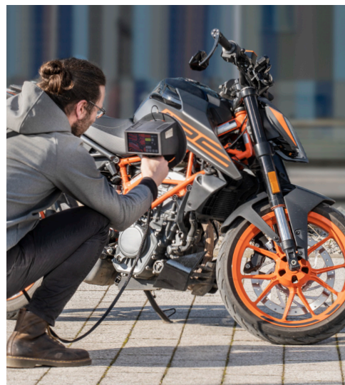
Simple capturing of a motorcycle with portable 3D sensor.
