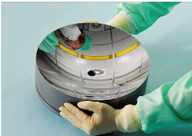
Coated EUV-collector mirror for high performance laser plasma sources used in lithography (Source: Fraunhofer IOF).
