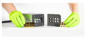
For comparison: The entire catadioptric optics take up only a fraction of a standard housing (shown here in gray) for conventional infrared cameras.
