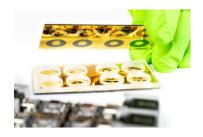
The new infrared camera uses an array of 2 x 4 sensors. The catadioptric mirror optics (shown here in gold) make the especially flat design possible. ©
