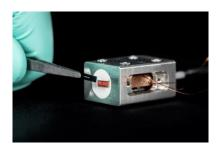
The housing of VCSEL laser diodes with integrated temperature control is extremely compact. © Fraunhofer IOF
