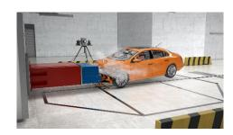
The goCRASH3D system uses two cameras (left and right) and powerful lighting (center) to capture up to 12,000 2D images per second, from which around 1,200 3D images are calculated. © Fraunhofer IOF In the crash test hall, several high-speed cameras record data from outside and now also inside the vehicle. © Fraunhofer IOF
