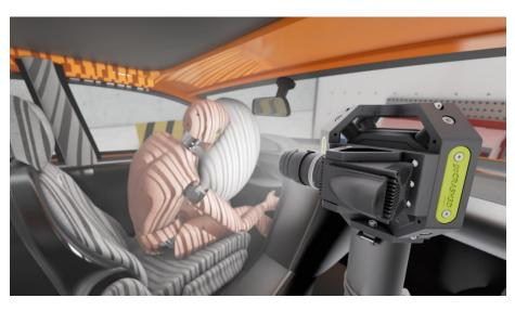
goCRASH3D (right) looks at the dummy with its cameras. The resolution of the two 2D cameras is 512 x 512 pixels each. © Fraunhofer IOF
