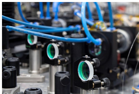
Laser output and mirror for beam guidance of three high-power laser beams. © Fraunhofer IOF
