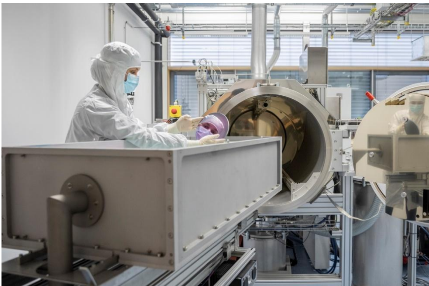
A researcher holds a highly reflective mirror for laser applications. The technology is to be optimized for laser fusion. © Fraunhofer IOF
